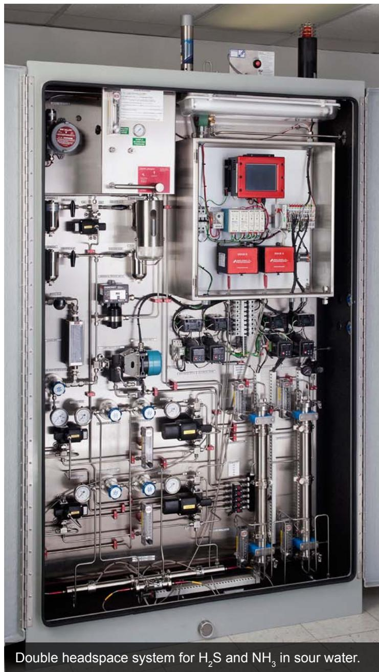
Double headspace system for H<sub>2</sub>S and NH<sub>3</sub> in sour water.
