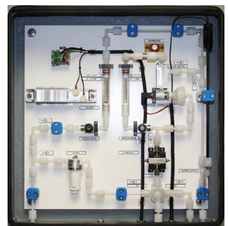
Ultra-Corrosive Sample SCS 0-50% Cl 2 and 0-30% NCl 3
