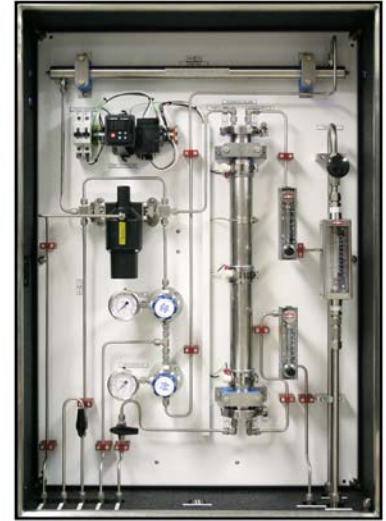
Headspace SCS 0-100 ppm H 2 S in crude oil
