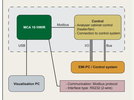
The system design consists basically of three logic units:
